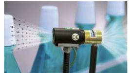
The Model 8294 Gen4 Ion Air Jet with Gen4 Power Supply neutralizes and cleans mouthwash bottles before heat shrinking the tamper-proof seal.
