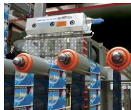
The Gen4 Super Ion Air Knife eliminates the static charge on labels being applied to PET soft drink bottles.
