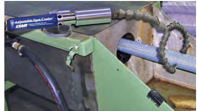
PVC hose is cooled at the exit of an extruder so it can be coiled immediately.
